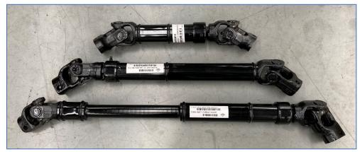
The only parts that should be replaced on a steering shaft is the end yokes & u-joints, anything else you need to replace the complete steering shaft.
